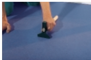
Hollow spots in the installation, rubbed-down linoleum covering can be „heard“ by running a hammer handle over the surface.
