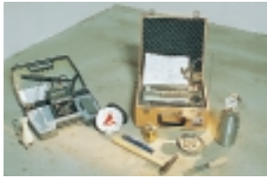
Testing the moisture content of the substrate and checking temperature and relative humidity in the room.
